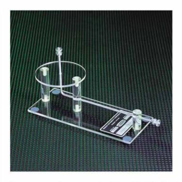
If we now move the compass to the 12:00 or 6:00 o'clock position, there is an immediate and large deflection of the needle. Another quick reference to the right hand rule shows the field around the conductor to be perpendicular to the normal direction of the compass needle. This field force will cause a deflection upwards of 45° and its direction will depend on which way the current is flowing in the rod.
